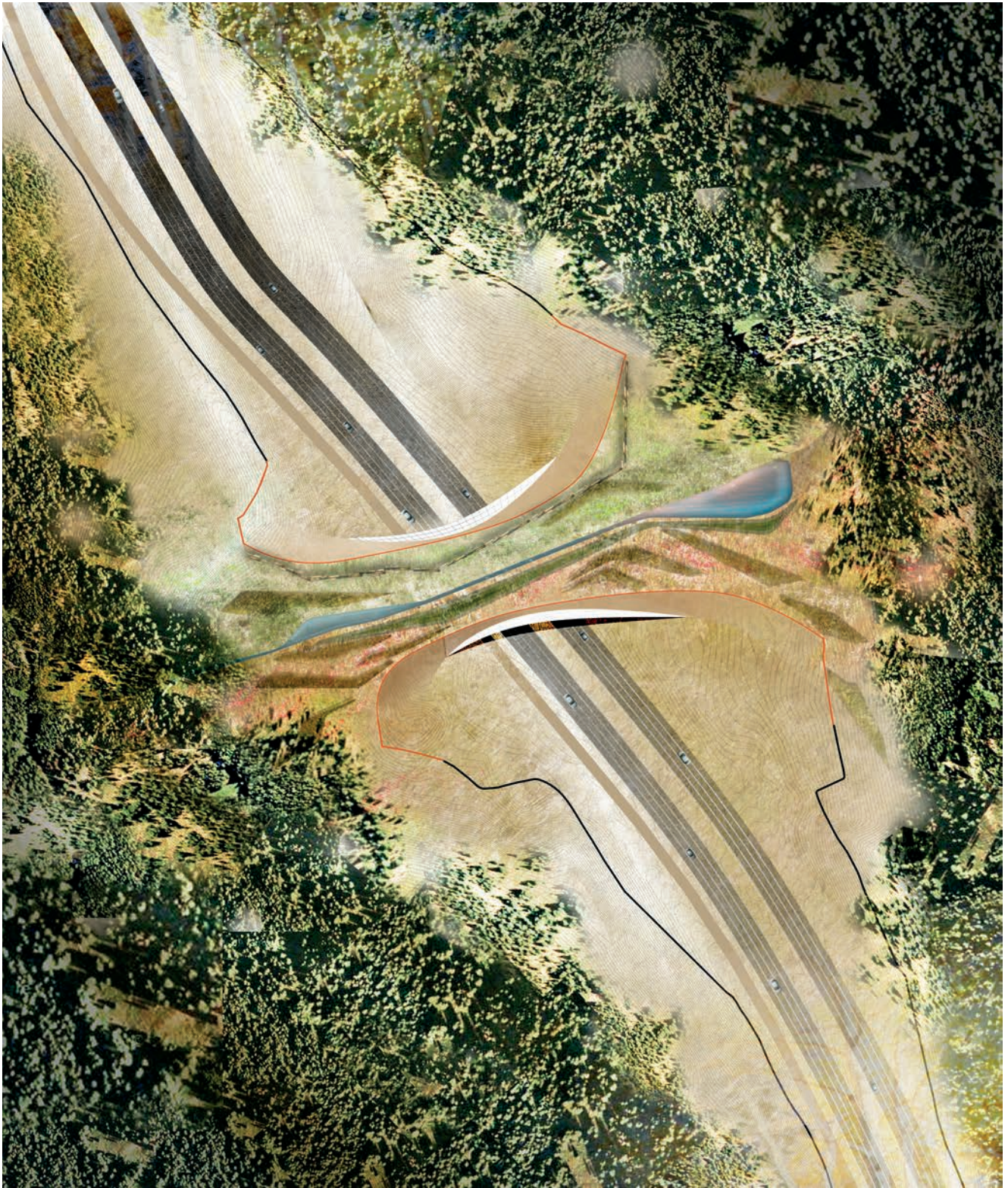
Figure 5. ARC wildlife crossing for Colorado, USA, showing connections to adjacent habitats and the proposed water channel in the middle of the crossing. © Zwarts & Jansma Architects and OKRA landscape architects.
